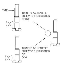
Fig. 5-2 A/C HEAD ASS'Y ADJUSTMENT (TILT ADJUSTMENT)
